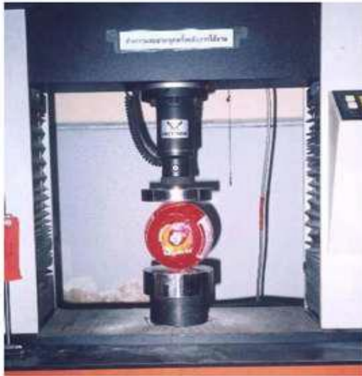
Figure 3- Pressure resistance test setup
